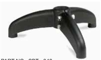
PART NO . SBT - 348 Material - Reinforced polyamide Hardware - Stainless steel Suitable tube - Ø48.3 mm Max applicable load - 10000 N
