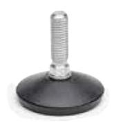
LEG PAD BASE (D)- 80,100,125 PART NO . **ALP - 1680,16100,16125** CUSTOM PART NO - **(AD)** Material - Reinforced polyamide Hardware - Stainless steel Max applicable load - 10000 N
